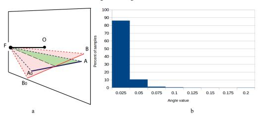
Figure 6. a. Illustration of two planes involved in error calculation. FO – the focal length of the camera (FO is normal to the frame plane), B0B - real road position, A0A - road position found by the algorithm.
