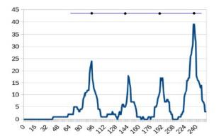
The line with bold points on the top represents a road pattern. Figure 4. The dependence of pixel intensities on the x-coordinate in the image.
